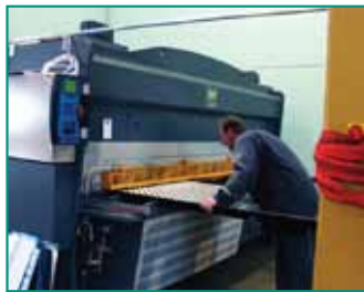
HACO plate shears 13mm/3000mm.
