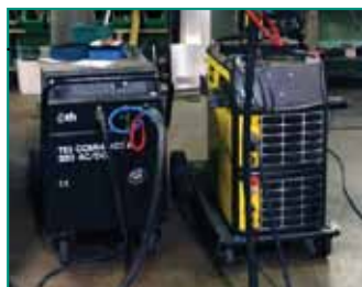
Welding units. Co2+TIG+ALU
