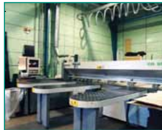
SELCO EB Saw, 95 mm saw for veneer, wood, plastic and fiber glass. 3,8 x 3,2 m x 80 mm with optimization.
