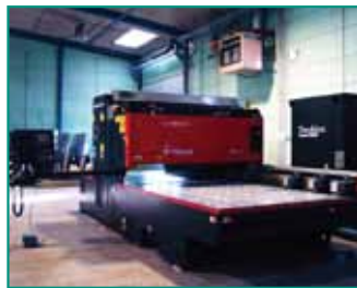
AMADA laser cutter 4kW 1500x5000x12mm.
