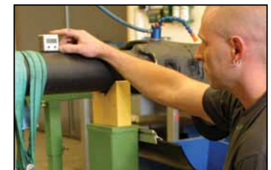
10 Control measurement of the axle.
